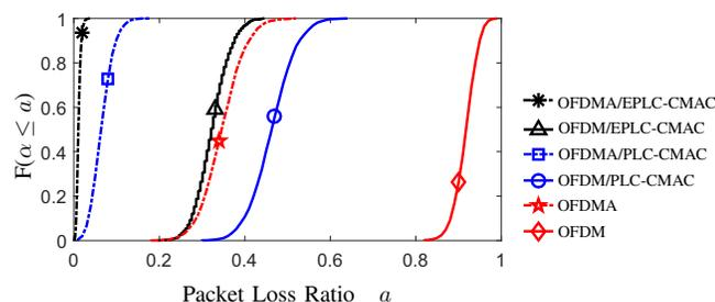
Figure 10: Packet loss ratio results considering the maximum correction of 1 bit per packet.
