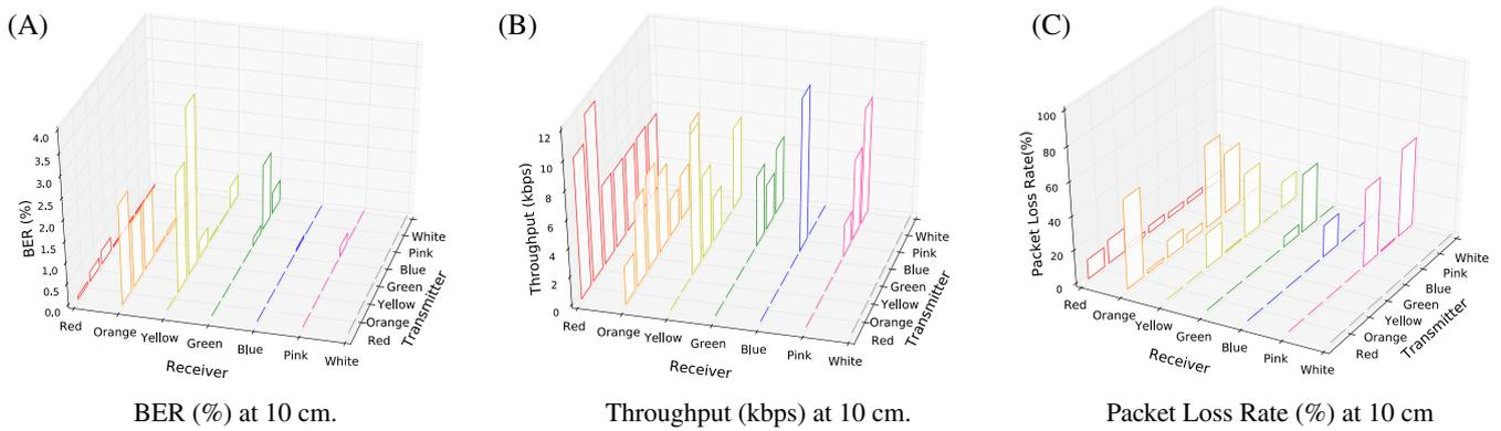
FIGURE 3 Bit error rate, throughput and packet loss rate for the combination of LEDs at a distance of 10 cm
