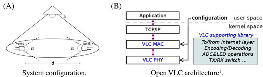
FIGURE 2 System organization and software architecture
