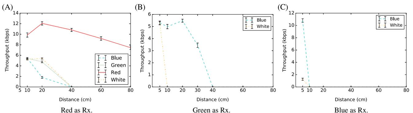
FIGURE 4 Throughput for LEDs of different colors as Rx
