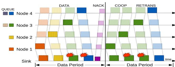
Fig. 3: Two frames of asynchronous COPPER in a 5-node scenario.
