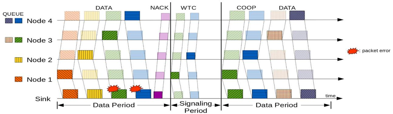
Fig. 2: Synchronous COPPER in a 5-node scenario.
