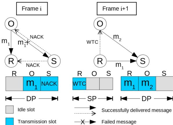
Fig. 1: Synchronous COPPER in a 3-node scenario.
