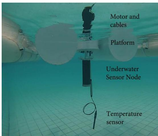
Figure 4: Underwater sensor node operating with a platform.
