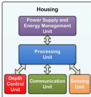
Figure 3: General underwater sensor node architecture.
