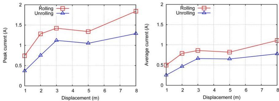
Figure 7: Energy consumption for depth control. Left: Peak current while moving the sensor. Right: Average current while moving the sensor.
