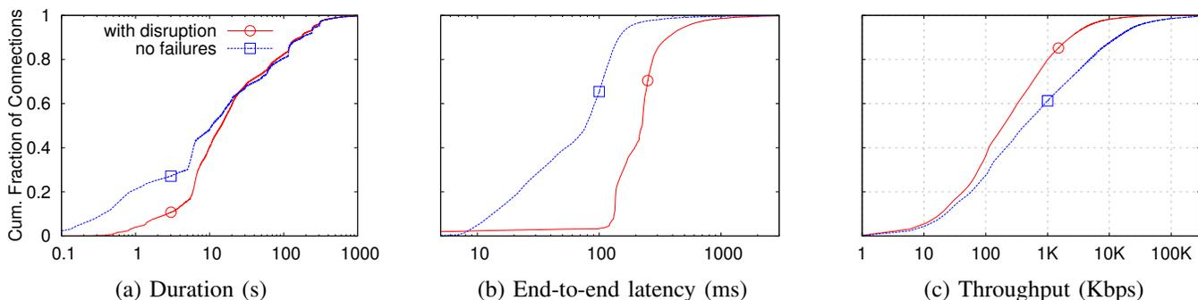
Figure 7: Performance comparison of TCP connections during the performance disruption on August 28th and the same period with no failure.
