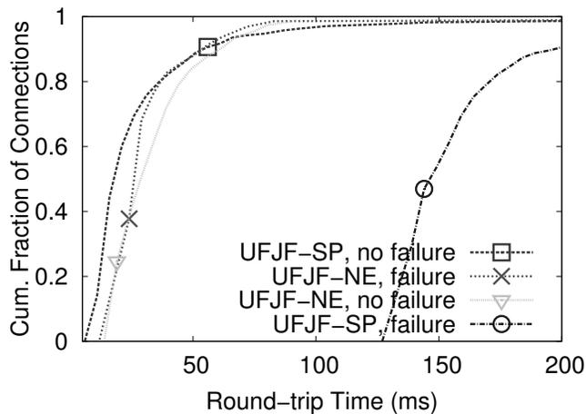
**Figure 9: Comparison of round-trip time between UFJF RNP exchange points located in São Paulo and Brazil’s northeast region for the reachability failure on August 28th.**
